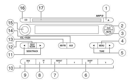
1. **CD eject:** Press to eject the CD/MP3.
